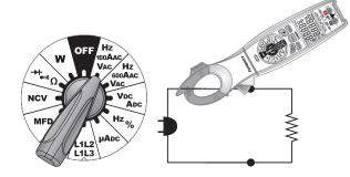
Amps AC (AAC), Frequency (Hz) through the clamp and Inrush AAC current is measured in the VAC/100AAC/Hz or VAC/600AAC/Hz switch position shown above.
