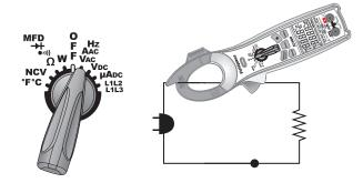
Amps AC (AAC), Frequency (Hz) through the clamp and Inrush AAC current is measured in the VAC/AAC/Hz switch position shown above.
