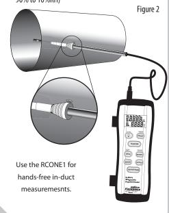
sure you do NOT drill a hole through any critical HVAC compo
