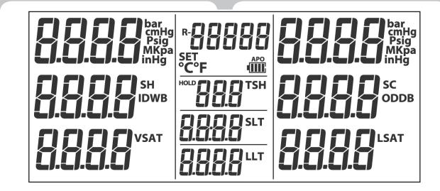
Pressure (bar) bar Psig Pressure (pounds/in<sup>2</sup>) Pressure (kilopascals or N MkPa inHg Negative Pressure (inche Negative Pressure (cm of cmHa SLT Suction Line Temperatur LLT Liquid Line Temperature VSAT Vapor Saturation Temper Liquid Saturation Tempe LSAT
