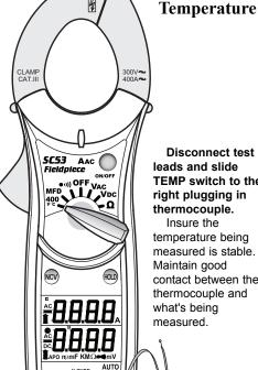
Disconnect test leads and slide TEMP switch to the
