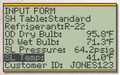
Figure 1. INPUT FORM for the Superheat test.
