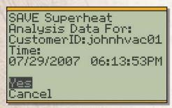
Figure 25. Saving data for Superheat analysis.
