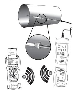
RCONE1 and AAT3 working with ET2W and HG3 to wirelessly log Wetbulb for target superheat testing.
